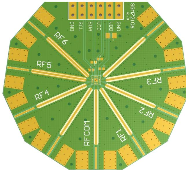
Figure 5. SGM72106 Evaluation Board Layout
