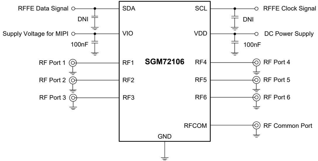
Figure 4. SGM72106 Typical Application Circuit
