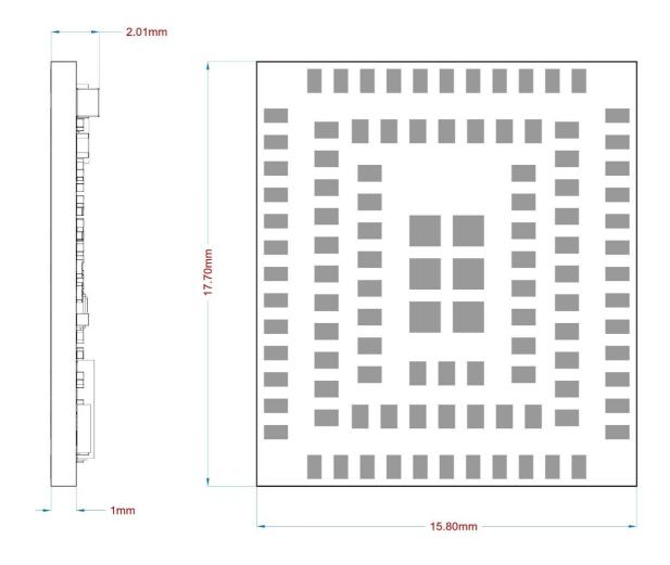
Figure 20: Front view and side view of the module (unit: mm)
