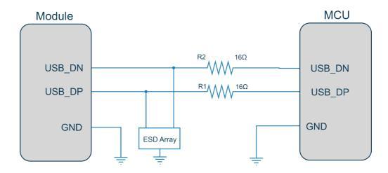
Figure 7: USB connection design circuit diagram
