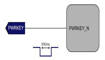
Figure 5: Power-on reference circuit
