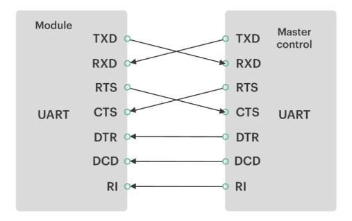
Figure 8: Full-featured serial port design
