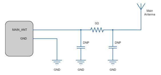
Figure 15: Main antenna matching circuit
