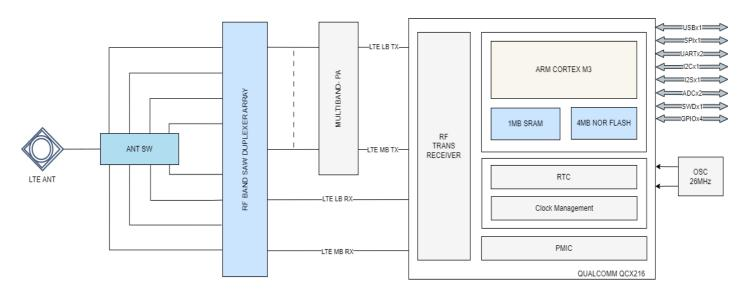
Figure 1: CQ16 Functional Block Diagram
