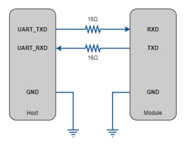
Figure 9: UART serial port design
