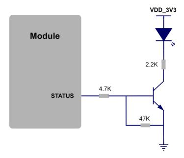
Figure 13:STATUS Pin Reference Circuit
