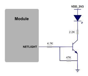
Figure 12: Net light reference circuit diagram
