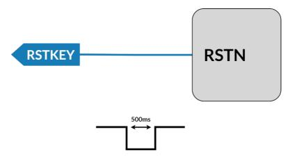
Figure 6: Reset reference circuit
