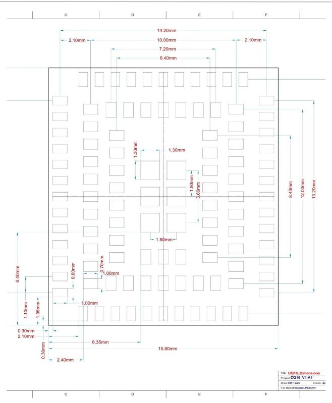
Figure 21: Bottom view of the module (unit: mm)
