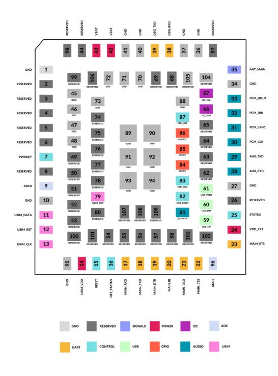
Figure 2: CQ16 module Interface definition (top view)
