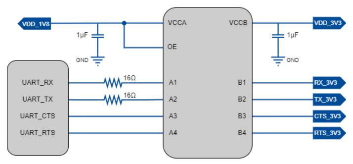
Figure 10: Level conversion chip circuit
