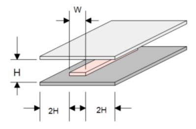
Figure 18: The complete structure of the multilayer PCB strip line
