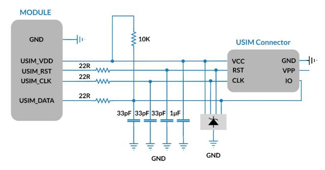
Figure 11: USIM design circuit diagram
