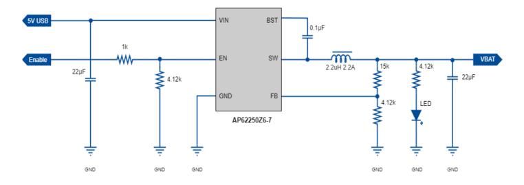
Figure 4: Buck converter reference circuit
