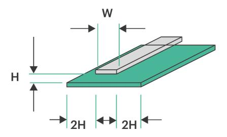
Figure 17: The complete structure of the two-layer PCB microstrip line
