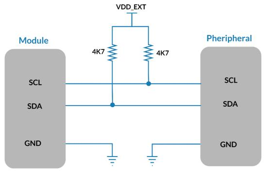
Figure 14: I2C interface reference circuit diagram
