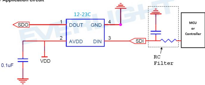
When 12-23C is set to operate on 5V power system, a 0.1uF capacitor is recommended to add between power supply and ground terminal. The capacitor is suggested to put as closer as possible to IC position. There are frequent resistors were used on different drain voltage as listed table.
