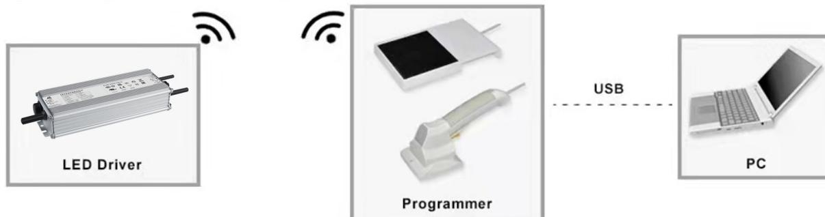
**Note:** The driver does not need to be powered on during the programming process.
