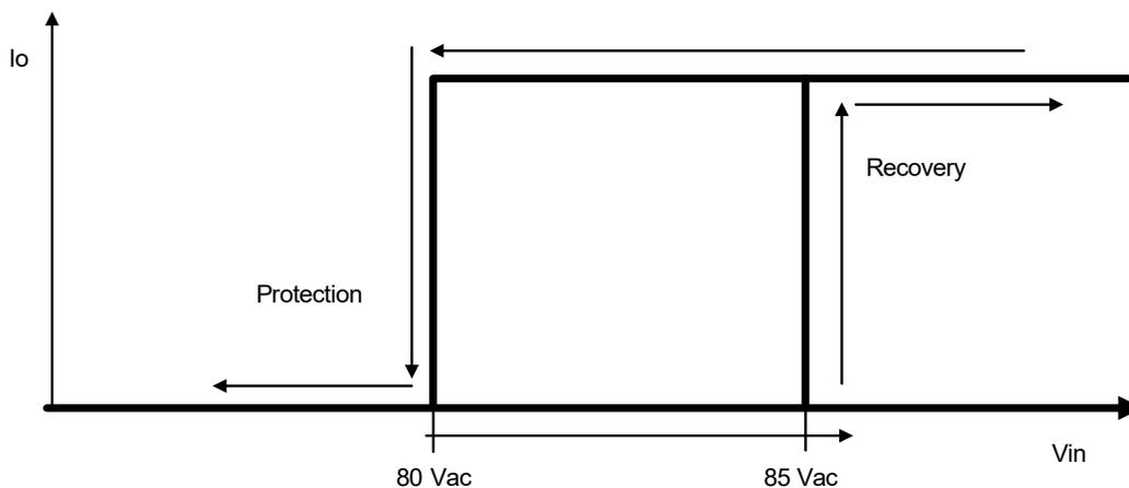
● **Input Over Voltage Protection Diagram**
