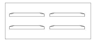
Do not stack LED drivers during installation. Keep a distance of at least 10cm between them to avoid affecting their heat dissipation and service life.
