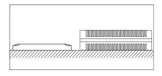
Don't directly contact the load with the LED driver during use. Keep a distance of at least 10cm between them to avoid affecting the heat dissipation and service life of the LED driver.
