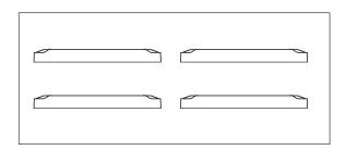
Do NOT stack drivers. Keep at least a certain distance between drivers when using them to avoid affecting the heat dissipation and lifetime of the drivers.
