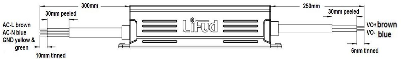
Cable specification: input 3\*17AWG/3\*1.04mm<sup>2</sup> (SJOW, H05RN-F) ØD8.2±1mm
