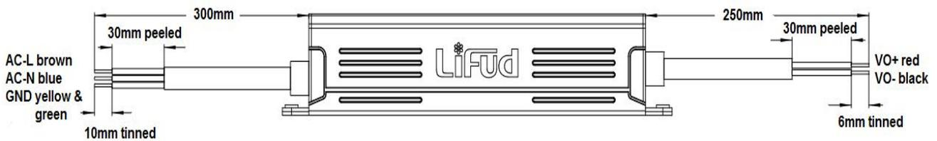
Cable specification: input 3\*17AWG/3\*1.04mm<sup>2</sup> (SJOW, H05RN-F) ØD8.2±1mm
