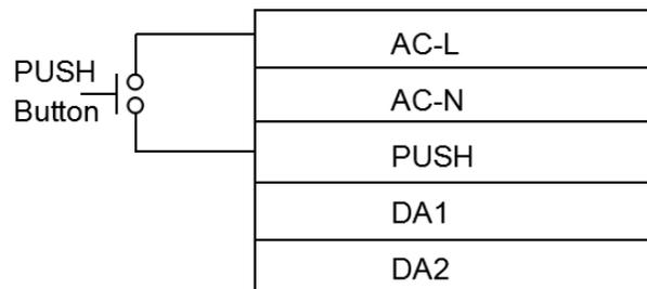
In the push dimming mode, double click (Each click is not less than 100ms. The interval of two clicks is not more than 200ms.) the push button and the dimming mode or the CCT changing mode will be switched to each other.
