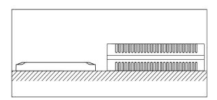
Direct contact between the load and the driver is prohibited when using the driver. Keep a certain distance between the driver and the load to avoid affecting the heat dissipation and lifetime of the drivers.
