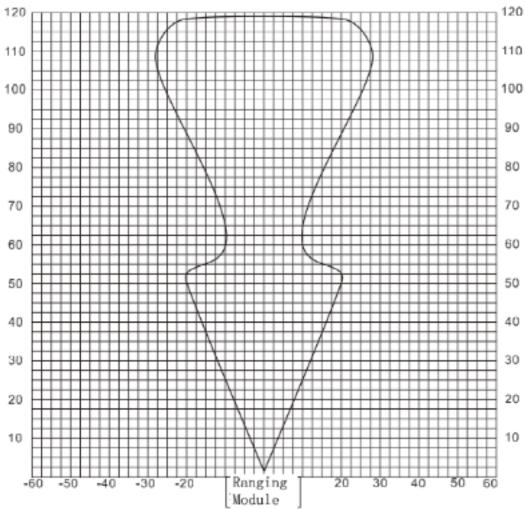
Notes: The area inside the curve is the area in which a 7.5 cm (diameter) circular rod can be detected.
