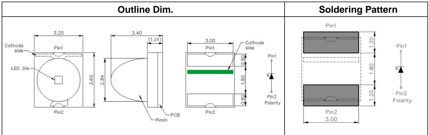
Soldering terminals may shift in the x, y direction.
