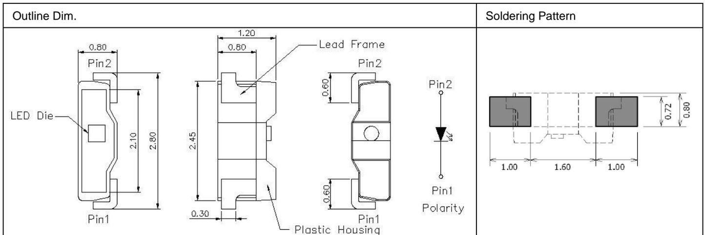
Soldering terminals may shift in the Wd direction.
