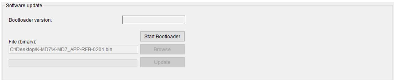
This tab allows the update of the V-LD1 firmware over the serial interface. The sensor starts to the application per default. The «Start Bootloader» button gives the option to start the bootloader out of the application.
