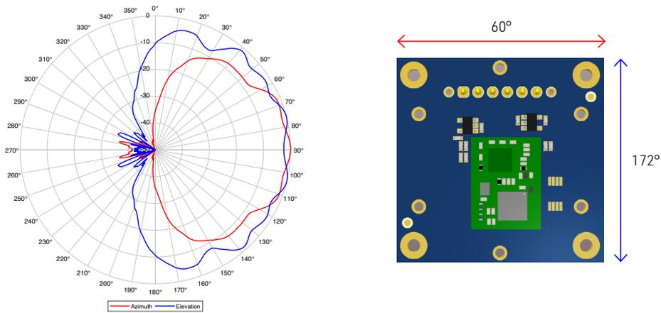
Figure 3: Overall antenna diagram with lens
