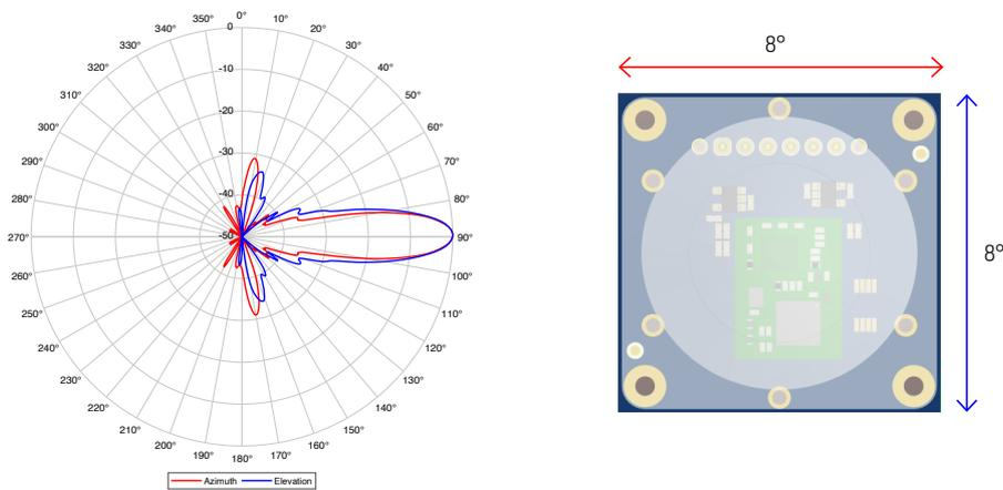
The lens can focus the beam width to about  $8 \times 8$  degrees and has a typical gain of 12 dBi. It is possible to integrate such a lens directly into the housing of a final product.
