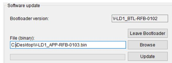
6. Wait until the process has finished. A message box indicates if the update was successful. The application starts automatically and by switching to the communication tab it is possible to directly connect to the sensor.
