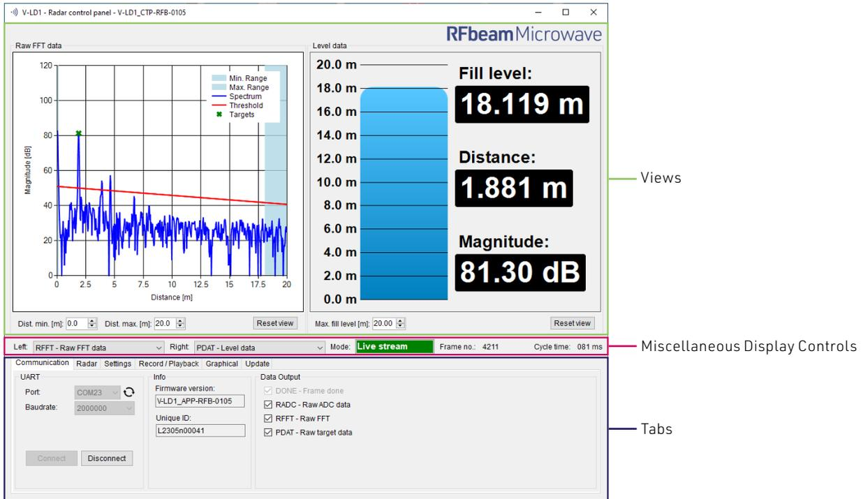
There are many views to select in the miscellaneous display controls area. All of them have a preceded shortcut based on the data output which is used in the views (RADC, RFFT, PDAT). To use the different views the according data output needs to be enabled.
