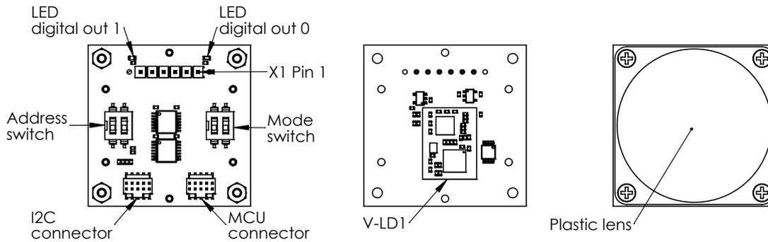
The V-LD1 evaluation kit consists of an evaluation kit PCB with a mounted V-LD1 in combination with a plastic lens which is mounted per default. The kit contains an FTDI cable which can be connected directly on connector X1 to power the sensor and create a virtual COM port connection to the PC.
