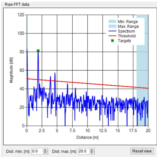
The RFFT view shows the range frequency spectrum in combination with the threshold. Furthermore the distance filter is visualised in this view.
